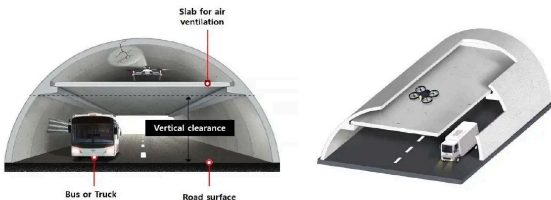
<Double deck tunnel: air ventilation space>
